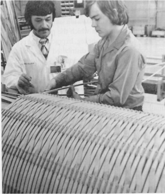
Figure 10.9c Primary winding of a large transformer; rating 128 kV, 290 A. (Courtesy ABB)
